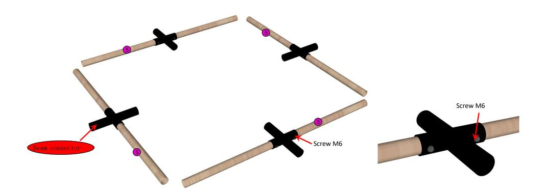
Step 4. Insert the assembled 5# poles into the inclined beam connection (there are reserved holes on the rod), and fix it with the hexagonal screws M6 (four sets in total), as shown below:
