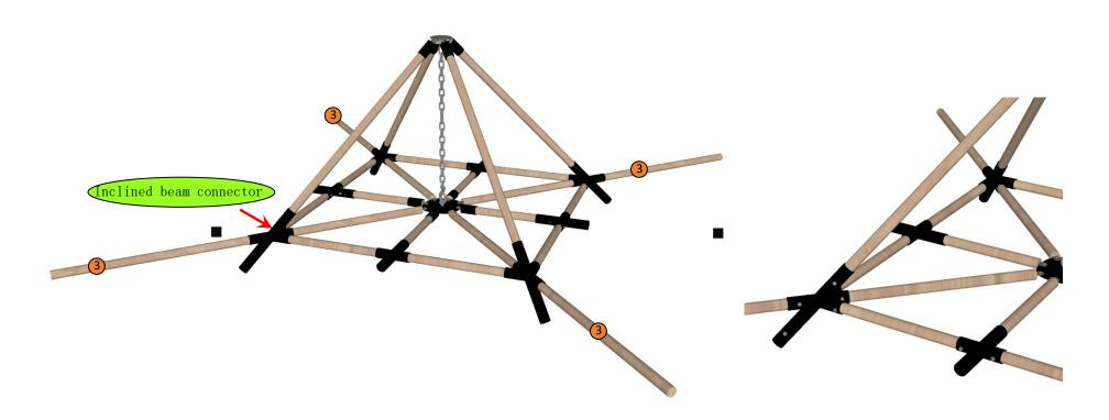
Step 8, Insert 1# poles into the connectors and fix it with hexagonal screws M6, as shown below:
