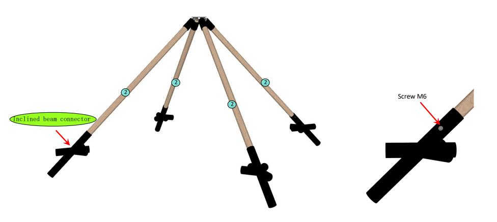
Step 3, Insert the 5# poles into the connectors assembly (there are reserved holes on the poles), and fix it with the screws M6 (four sets in total), as shown below:
