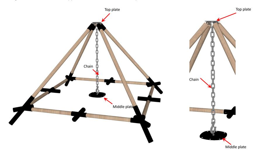
Step 6. Insert one end of the 6# poles into the connectors, and connect the other end to the middle plate, and fix them with screws M6 and M20\*40 respectively, as shown in the figure below.:
