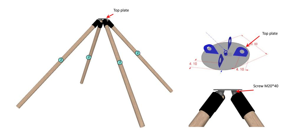
Step 2, Insert the inclined beam link into the 2# poles (there are reserved holes on the pole), and fix it with the screws M6 (four sets in total), as shown below:
