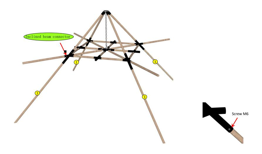
Step 9, Insert the bases into the 1# pole and fix it with the external hexagonal screw M6; fix the bottom where it meets the ground with the Self-tapping screw (stainless steel) M8\*60, as shown below:
