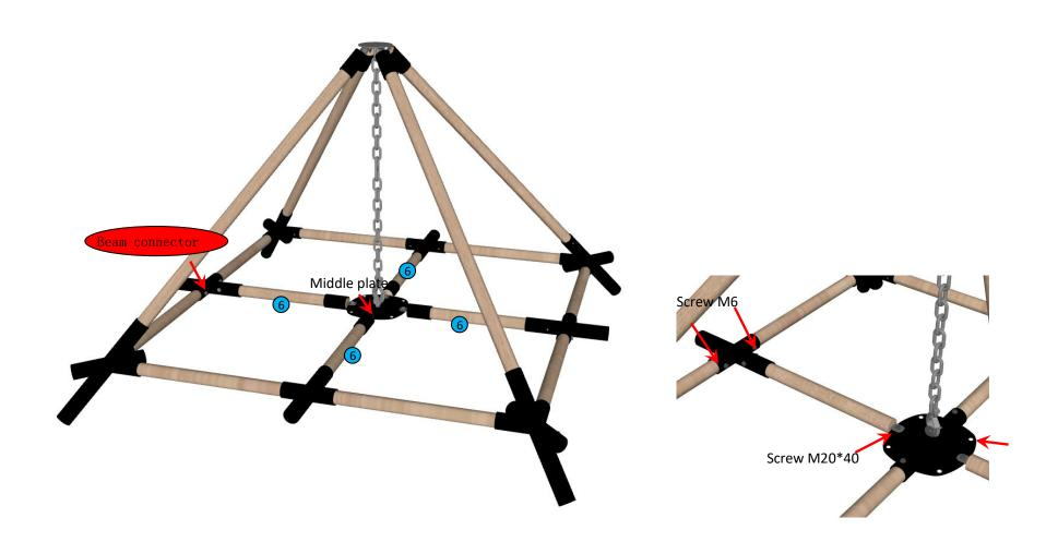
Step 7, Insert the 3# poles into the inclined beam connector and assemble it with the middle plate, and fix it with the hexagonal screw (stainless steel) M20\*40, as shown below:
