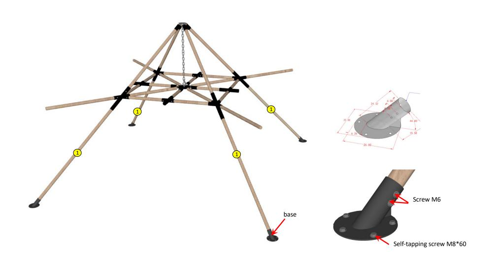
Step 10. Insert the 4# poles into the connectors and fix it with the screw M6, as shown below:
